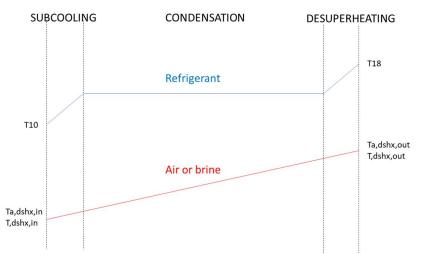
Figure 12. DSHX working as a condenser (Cooling mode). Refrigerant can exchange heat with air, brine or both at the same time.
