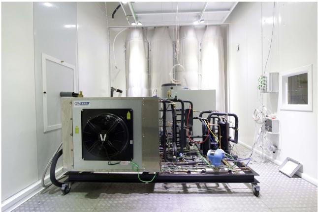
Figure 9. DSHX test bench installed inside the climatic chamber.
