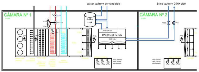
Figure 8. Scheme of the DSHX test bench installed in the climatic chamber.
