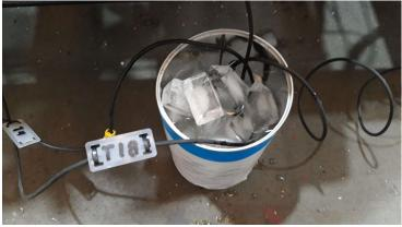
Figure 1. Temperature sensors submerged in iced water.
