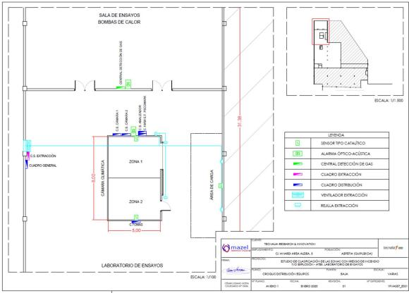
Figure 5. Drawing of Tecnalia's laboratory Layout.
